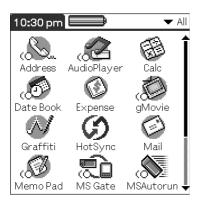
As well as being your gateway to all the applications, the **Application Launcher** screen displays the current time, battery level, and application category.
